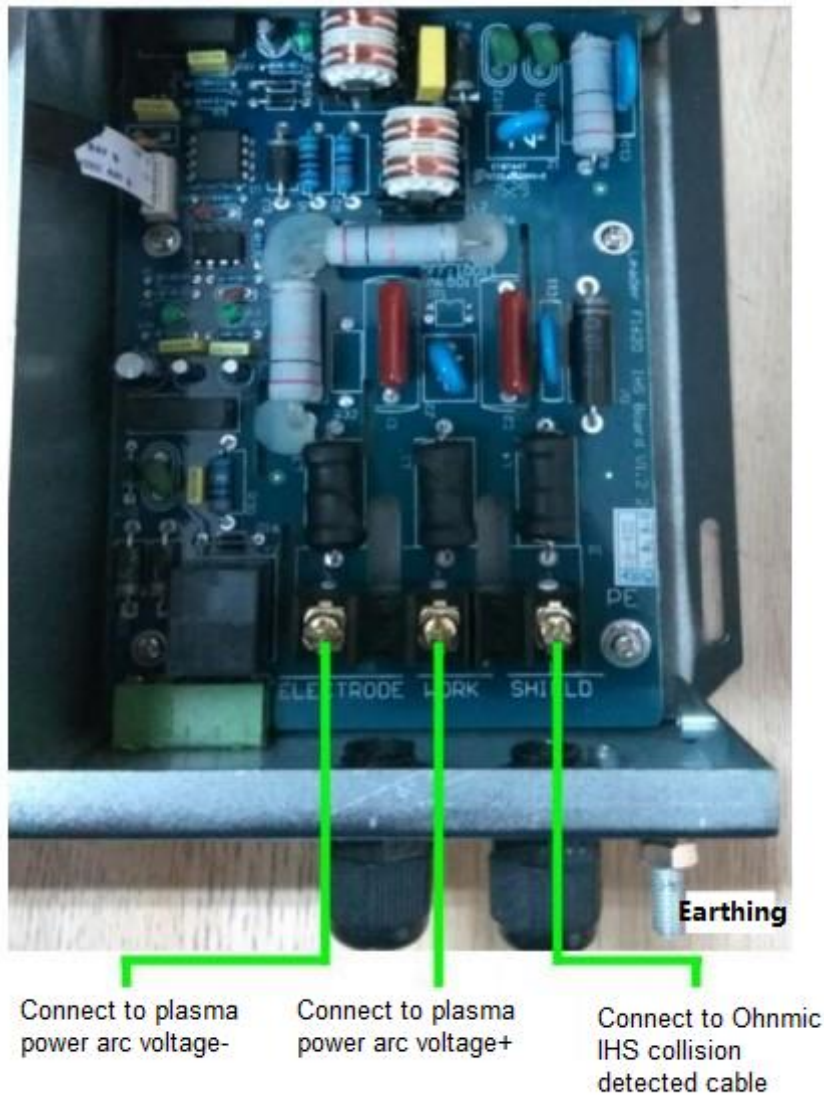
Figure 3.9 Connection of voltage divider Interface
